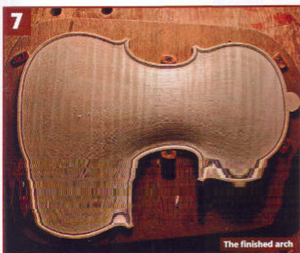
Building the facets of the arch
